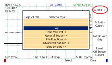
This will change horizontal scale settings so your cable trace is nicely sized on the screen. If your cable is actually longer than the Short length limit, it will automatically reset to Medium length.
