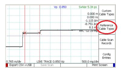
Or you can set the Vp manually. If the Vp value is not displayed in the top-center of the screen, press the M-FUNC button until it is. Now adjust the Vp value by turning the M-FUNCTION knob.
