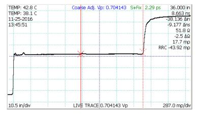
We can use the VERTICAL and HORIZONTAL SCALE knobs to zoom in on the connector. The three bumps each measure one of the connections: from BNC cable end to BNC barrel, then from BNC barrel to the adapter, and finally from the adapter to the SMA cable.
