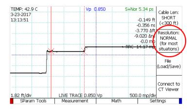
Normal resolution allows the CT100B to perform at a relatively high rate of speed while still generating detailed scans over long cable lengths. It is a convenient default setting that you can use except for special circumstances.
