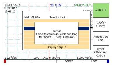
The result is scaling that allows the whole cable trace to be visible. The cursors are positioned at the beginning and end of the cable. The picture below shows a cable that is about 1000 ft long that is "open" at the end.
