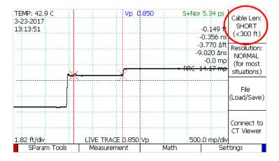
If you are not sure of the length, you can start with the Short setting. Running Autofit (described in the next step) will increase the length setting if necessary.
